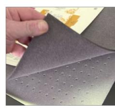
Vacuum hold down table. Sheets are held securely in place on either a green self-healing or superior grey felt cutting mat, by a vacuum produced by a powerful centrifugal air pump. Suction passes through the perforated hold down table and the mat, keeping sheets flat and secure.
