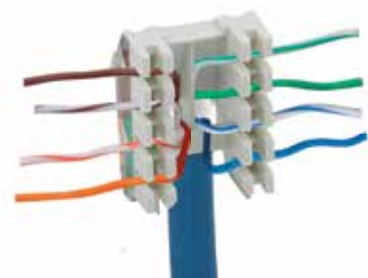
2 Separate and fit the pairs
