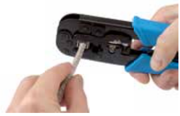
3/ Crimp to complete the connection
