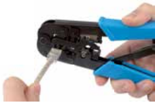
2/ Place the connector in the tool
